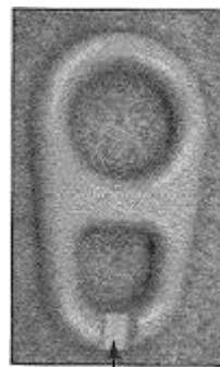
Figure 18. The flat link has a notched section of plastic, which breaks when a force of 600 pounds or greater is applied to it.
